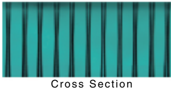
▲ Dia.: 25 μm, thickness: 500 μm, silica glass
